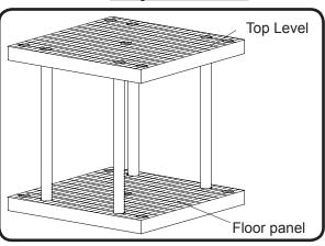
Insert (4) 36" legs into Floor Panel (open hole socket)
