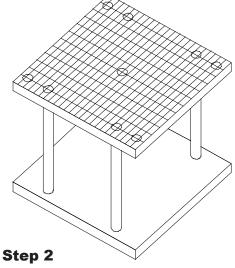
Next, slide (1) Top Panel (closed hole sockets) on 36" legs. Make sure panel is pushed all the way down as shown.
