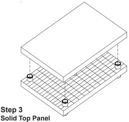
Next, align the sockets of the **Solid Top Panel** above the **Stackers** and push panel all the way down until resting on the **Grid Panel** as shown. (Make sure the panels are pushed together tightly).
