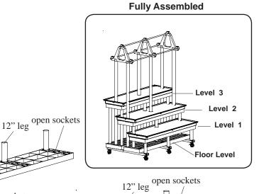
Step 2 12" Legs Level 1 Position the Level 1 Panel on 12" legs overhanging outside edge. Next, position Level 1 waterbed (open holes) on level
