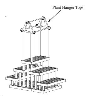
Step 7 **Plant Hanger Assembly** nsert Plant hange assembly in 72" legs as shown.
